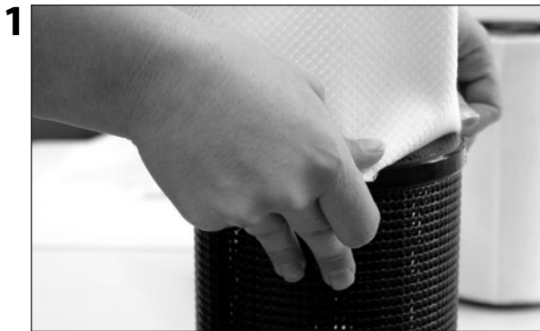
Pull a post-filter sleeve over each of the cartridges. With new IQAir systems the sleeves are supplied inside of the IQAir System (refer to Chapter 2 on how to open the IQAir System).
